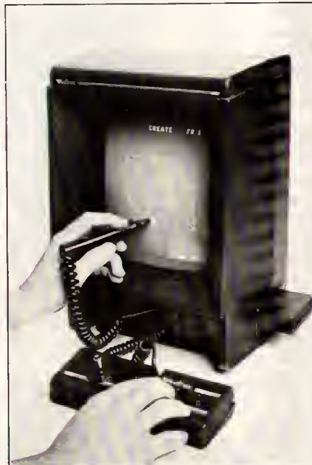
True interaction comes to the vector graphics Vectrex system with the introduction of a light pen.
